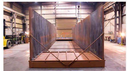
Collapsible Bulk Storage Tank with both side walls up and in place.
