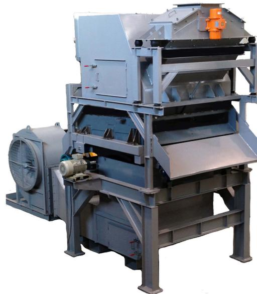
**Densimetric Tables are designed to separate materials through material density, typically of a dry product. They have successfully been used to separate a wide array of materials for industries, including various recycling, mining, and food and beverage applications.**
