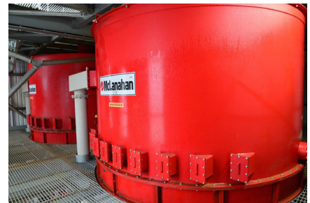
Side removable teeter water pipes eliminate the need for entry into confined spaces to perform routine maintenance.
